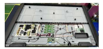
And then remove cabinet & speakers with hand and screw driver.
