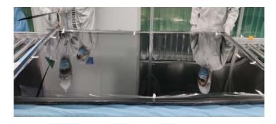
LCD module(together with their casing) is only left after all other parts like electronic units and casing have been removed.
